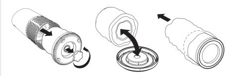
Unscrew knob, loosen bottom cover, and remove plastic bag from filter.
