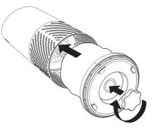
Secure filter on bottom cover, slide both into purifier, and reattach knob.
