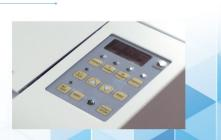
Easy to operate digital panel. Set start and stop and number of sheets easily and quickly on the digital LCD operation panel.
