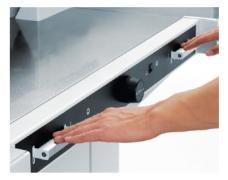
Easy cut blade activation bars require two-hand operation and allow blade & clamp to perform independently
