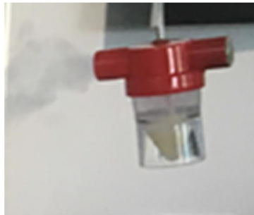
Figure 2. The nebulizer used to generate the microbial inoculum.
