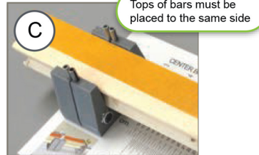
C. 1500 Standard Extending a bar Place bars with the tape to the outside making sure that the tops of the bars are on the same side.
