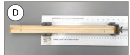
D. 1500 Pro Place bar with tape to the bottom. Pro bars are cut one at a time regardless of extending or shortening.
