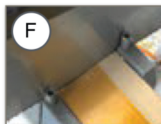
F. Place saw between the metal guiding posts and proceed to cut with a steady back and forth motion.
