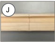
J. Cut ends of bars together.
