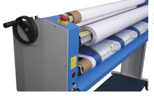
Integrated Rear Rewind makes Roll-to-Roll applications easy.
