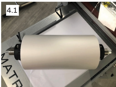
4. Slide film onto the mandrel and centralize (4.1). Replace the core adaptor and tighten. Place the mandrel back onto the system and tighten the mandrel lock (4.3).
