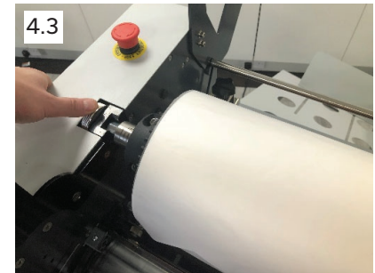
4. Slide film onto the mandrel and centralize (4.1). Replace the core adaptor and tighten. Place the mandrel back onto the system and tighten the mandrel lock (4.3).
