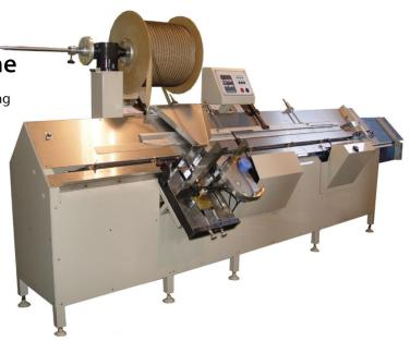
documents per hour. As the operator, you simply set up your job using the control panel, place the documents to be bound onto the left side of the machine, and watch the unit do the rest; jogging the sheets, cutting the wire to length, inserting the wire, closing the wire, and dispensing the finished books onto the exit conveyer for easy handling.
