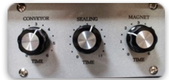
Sealer Control Panel
