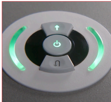
i-Control Switch with Dynamic Load Sensing and other status indicators
