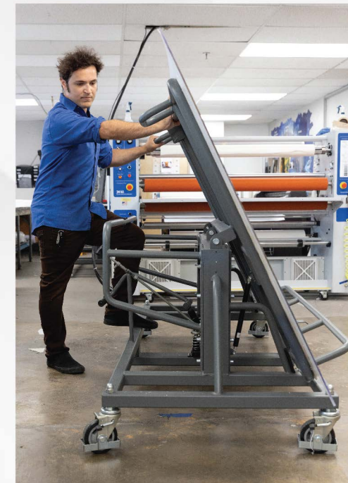
The tilt down and locking feature lets the operator safely move heavy rolls from horizontal to vertical position.
