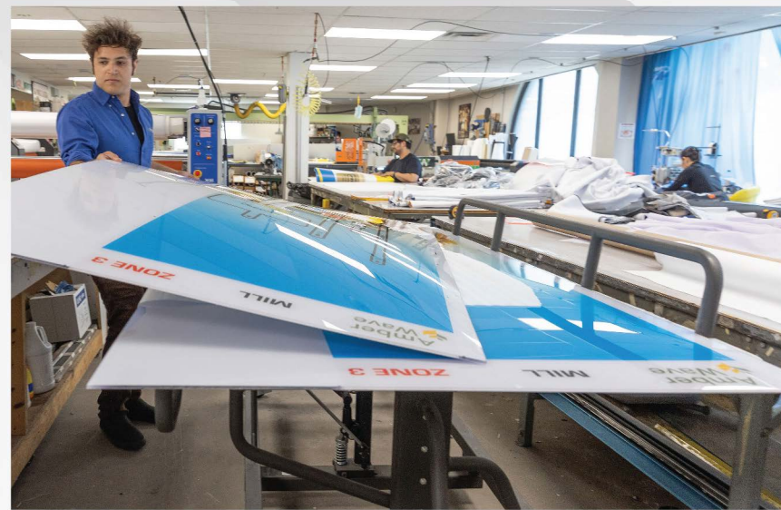
Deck rails keep 8" stacks of rigid substrates from shifting and moving during transport and loading.
