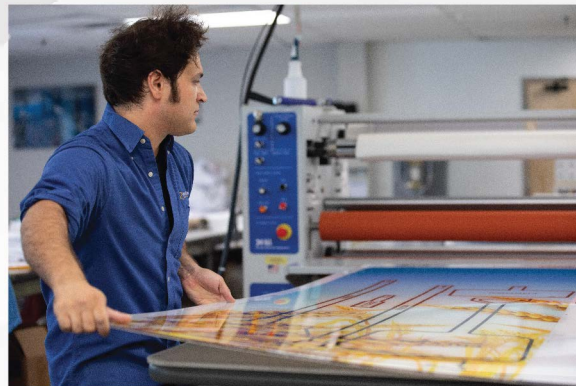
Operators can quickly and safely feed boards onto printers, cutters, and laminators without bending or lifting.
